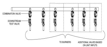
FIG. 29 Typical Boiler Gas Train Drawing
